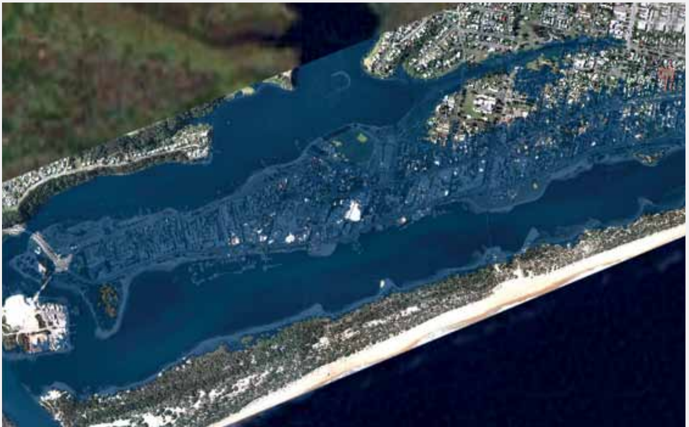
Figure 2. Lakes Entrance with simulated coastal flooding of 180 cm above sea level.
